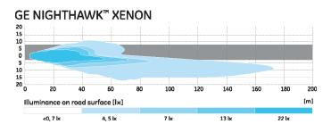
\*GE NIGHTHAWK™ XENON headlamps focus more light on the road - flux projected to area with more than 15,000 candelas in light intensity compared to a standard halogen headlamp bulb. Specific light levels vary by bulb type and headlamp assembly.
